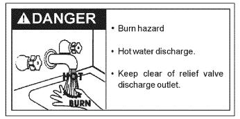
The temperature-pressure relief valve must be manually operated at least once a year. Caution should be taken to ensure that (1) no one is in front of or around the outlet of the temperature-pressure relief valve discharge line, and (2) the water manually discharged will not cause any property damage or bodily injury. The water may be extremely hot.
